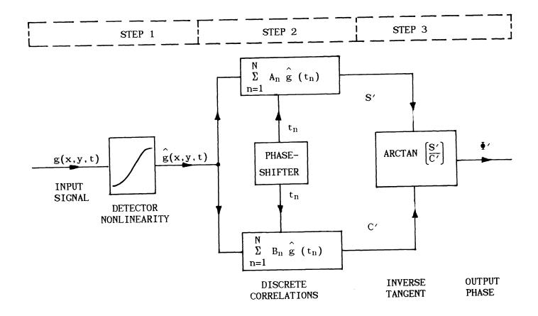
Figure 1. Phase-shifting process - schematic
