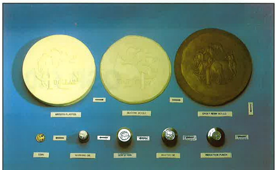
Range of tools used in the minting process. All can be measured by the OSP 130
