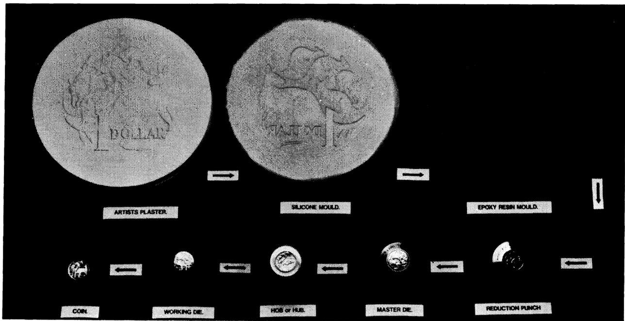
Figure 1. Range of tools used in the coin minting process.
