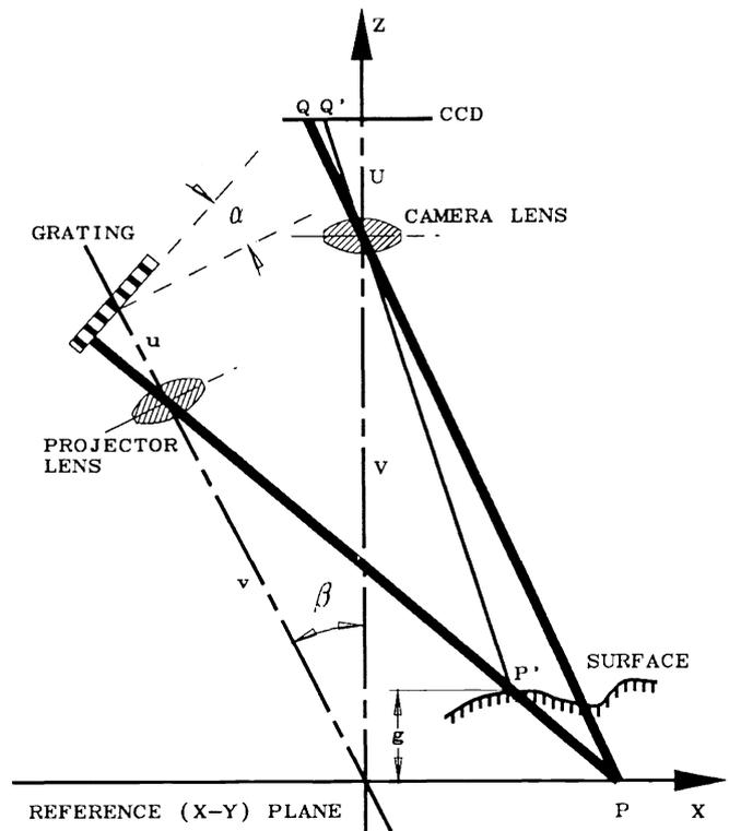
Figure 3. Schematic of the OSP130 projection and observation geometry.
