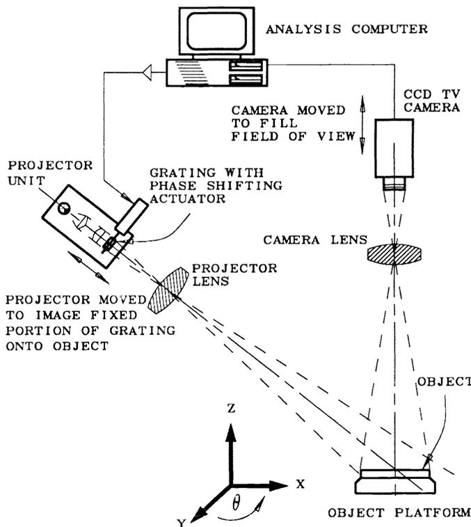
Figure 2. Functional schematic of the OSP130 instrument.
