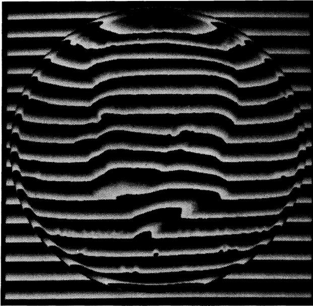
Figure 6. Grating phase map for a half dollar USA Coin (JFK side).
