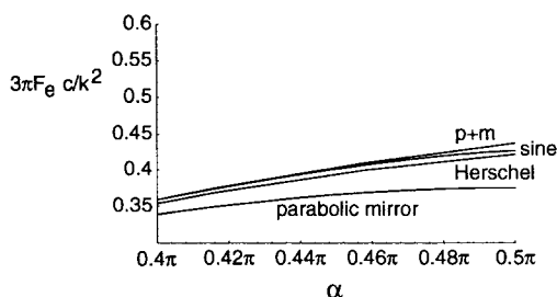
Figure 4. The ratio of the electric energy at the focus to the incident power, as a function of the angular semiaperture \alpha for various different conditions. A system obeying the sine condition behaves very similarly to the mixed-dipole field.
