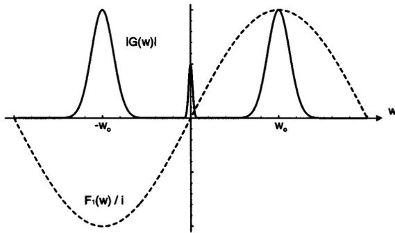
Fig. 2. Modulus of the Fourier-transformed correlogram,  $|G(w)|$ . The normally large dc term has been reduced in magnitude to fit within the chosen scale. Also shown for comparison is the FT  $F_1(w)$  of the finite-difference filter  $f_1(z)$  with separation  $\Delta = 1/4w_0$ .
