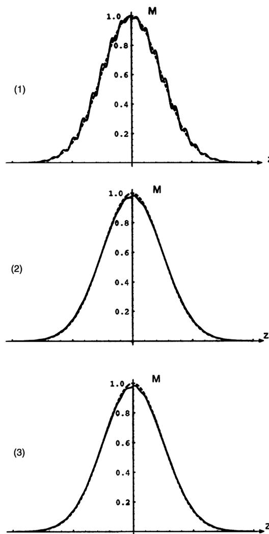
Fig. 4. Envelope detection for all three algorithms with use of a  $90^\circ$  step size. In this particular case the curves produced by algorithms (2) and (3) are the same. Algorithm (1) has noticeable fringe structure.
