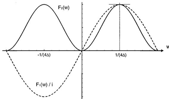
Fig. 3. FT's  $F_1(w)$  and  $F_2(w)$  of the five-step phase-shifting filters  $f_1(z)$  and  $f_2(z)$ . Note particularly the stationary points at  $w = \pm 1/4\Delta$ .
