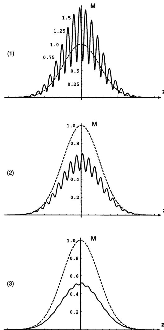
Fig. 6. Envelope detection for all three algorithms with use of a  $135^\circ$  step size. Again both algorithms (1) and (2) have significant fringe structure visible, whereas algorithm (3) shows only a trace of the second-harmonic fringe structure.
