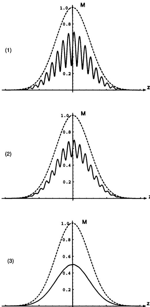
Fig. 5. Envelope detection for all three algorithms with use of a  $45^\circ$  step size. Both algorithms (1) and (2) have significant fringe structure visible. Algorithm (3) performs exceptionally well and has a 50% reduction as predicted.
