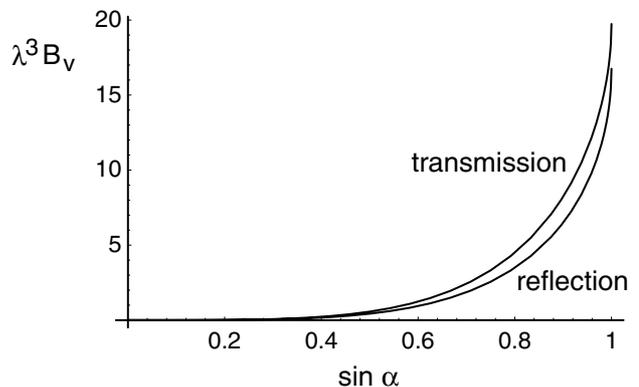
Fig. 1. The volume of the three-dimensional coherent transfer function (CTF) of confocal transmission and reflection systems, as a function of  $\sin \alpha$ .
