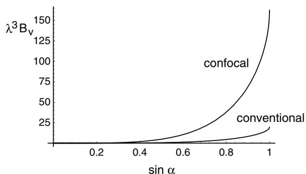
**Fig. 2.** The volume of the three-dimensional optical transfer function (OTF) of conventional and confocal fluorescence systems, as a function of  $\sin \alpha$ .
