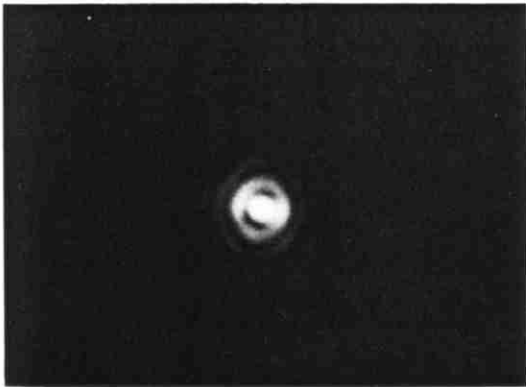
FIGURE 6. The (indirect) image of an illuminating spot obtained by placing a CCD camera at the detector plane of a confocal microscope with the scanning mechanism turned off. A front-surface mirror was used as a specimen.
