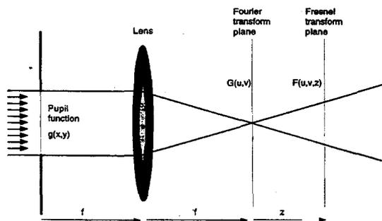
Figure 3 Fraunhofer and Fresnel Diffraction
