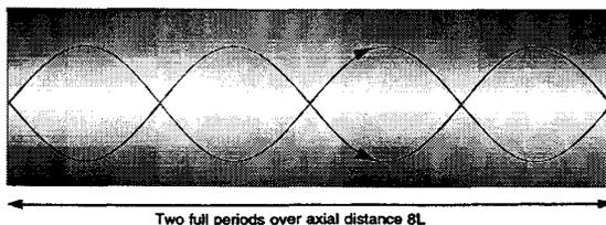
Figure 1 Ray propagation in a GRIN medium
