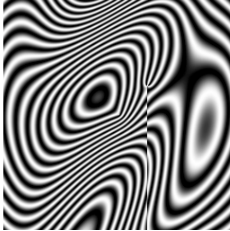
Fig. 4. Fringe pattern used for testing the phase-shift calibration algorithm. Note the closed fringes, the rapid fringe spacing variation and the fringe discontinuity – factors which defeat many other techniques. The sampled intensity varies between 0 and 255 grey levels.
